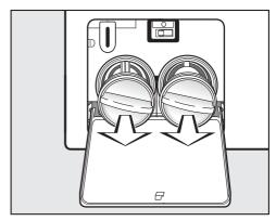
■ Remove the drain filters completely.
